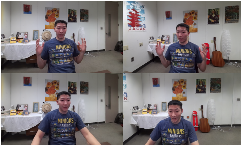
Figure 1: We present a capturing and rendering system designed for personal telepresence. (left) Our system utilizes four RGBD cameras to render high-resolution free-viewpoint videos, which are crucial to immersive 3D video conferencing. (right) We show synthesized images from different novel viewpoints across different frames.
